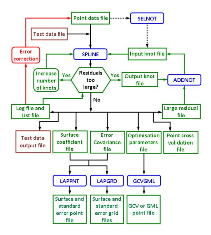
Figure 1. Main data flows through the ANUSPLIN package. The procedure for choosing and updating knot sets is described in a following section. Knot selection is also demonstrated in the provided annotated examples.
